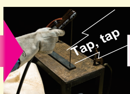
When restarting work, tapping the base metal with the electrode.
