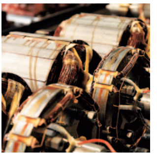
Varnishing of rotors for protection against earthquakes, corrosion and harmful substances
