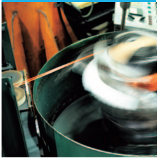
Winding of copper wire to the rotor by an automatic winding machine
